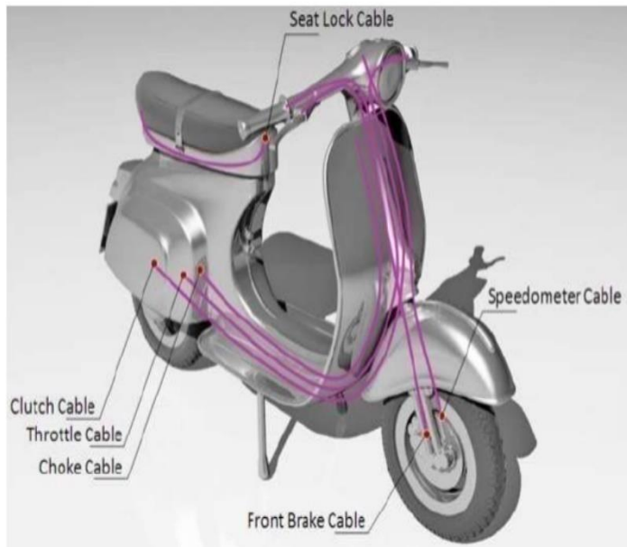
Exhibit 63: Cables in 2Ws
